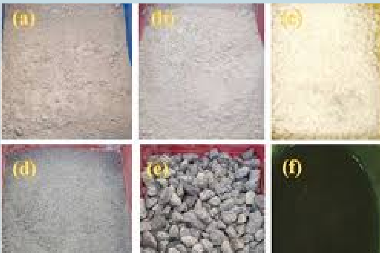
Fig. 3.1 Raw materials used for PPFRGPC preparation, (a) fly ash, (b) GGBS, (c) NaOH pellets (d) fine aggregate, (e) Coarse Aggregate, (f) Na 2 SiO 3 Solution.
