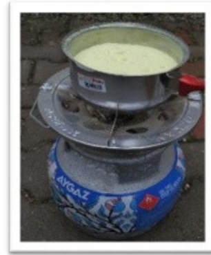
Fig. 3 Heating of sulphur and providing binder feature
